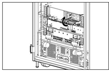
Figure 1-2: Unlocking the server blade from the enclosure
